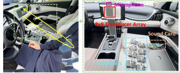
Fig. 12: DASIV deployment in the vehicle.
