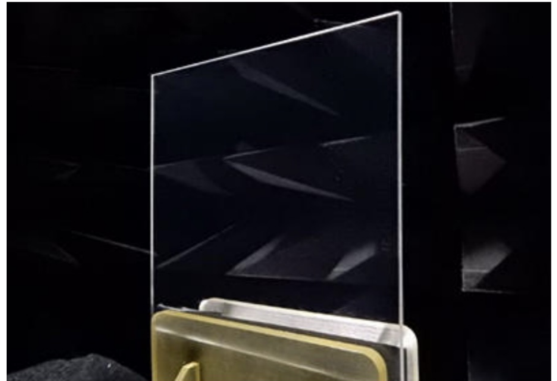
Transparent Transmissive Metasurface (Prototype)
