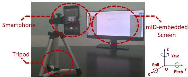
Fig. 12. Current page of the display is embedded with mID, which can be captured by the built-in cameras of smartphones.
