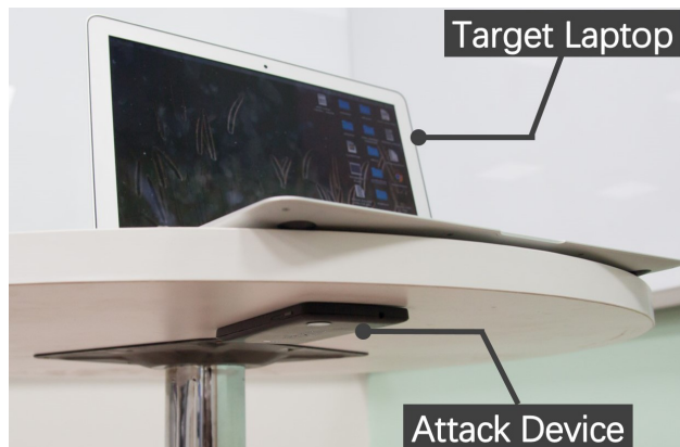
Fig. 7: The experimental scenario of MagAttack. We keep the attack device under the table to draw no attention. The round table is 2.5 cm in thickness.
