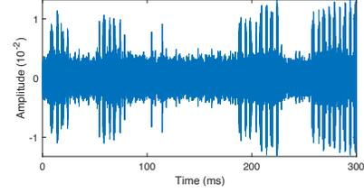
(a) Modulate the leakage current with the preamble and the binary sequence.
