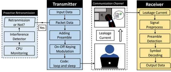
Figure 4: System architecture of the *TouchHBC* system.
